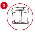
Lock The Bowl Turn clockwise to click the bowl into the locked position.
