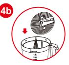
Mount The Disc When using a blade disc, insert the driving shaft, then put assembled disc holder and disc blade together into the bowl.
